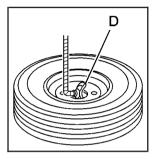
2. Tilt the retainer (D) downward and through the wheel opening. Make sure the retainer is fully seated across the underside of the wheel.
